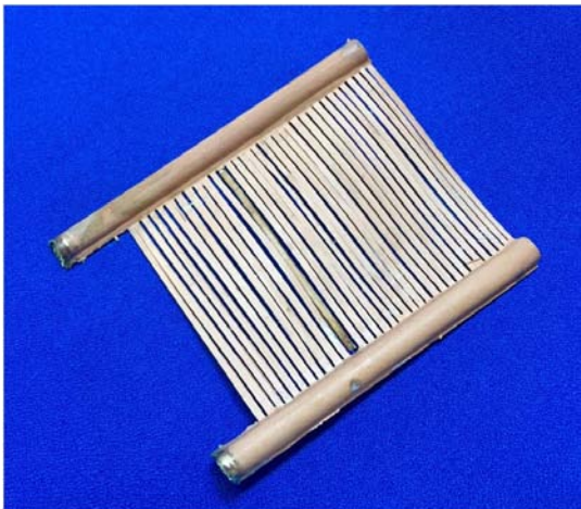
Figure 9. Micro-channel array measuring 5 cm x 5 cm and weighing 1.8 g
