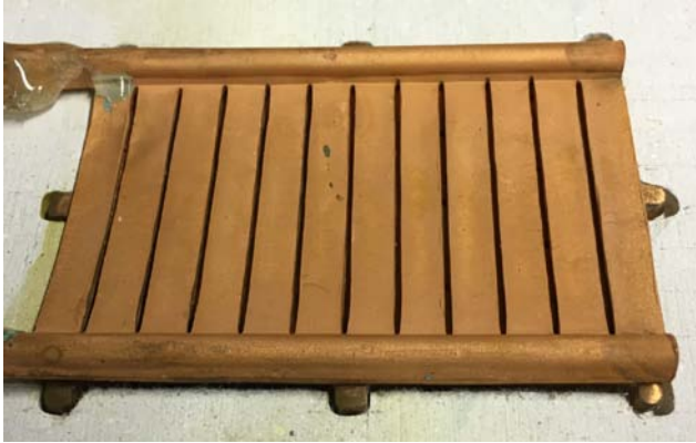
Figure 18. 12-Channel thermal management unit produced using the additive-based manufacturing process
