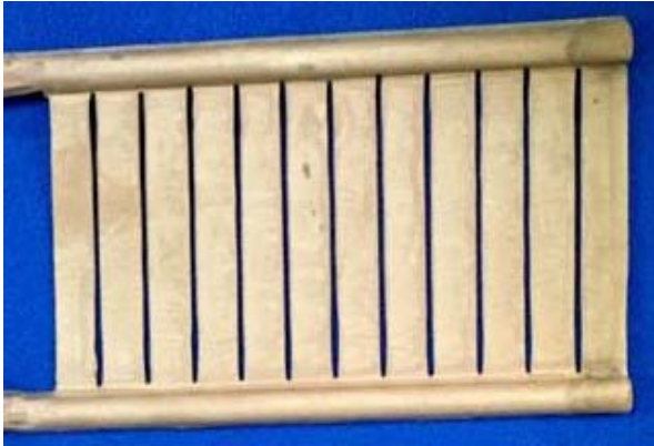
Figure 7. Liquid-cooled multi-channel array measuring 5 cm x 7.6 cm and weighing 6 grams
