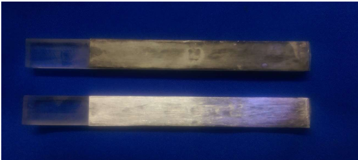
Figure 12. Silver electrodes that have been in the biocide generator operating for 8 hours; the top electrode is untreated, while the bottom electrode has undergone three minutes of abrasion cleaning
