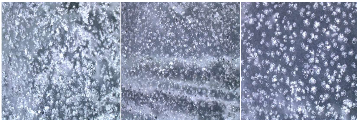
Figure 7. 5.4 mil filler particles at ratios of 6:1, 10:1 and 16:1 (Nafion:filler)
