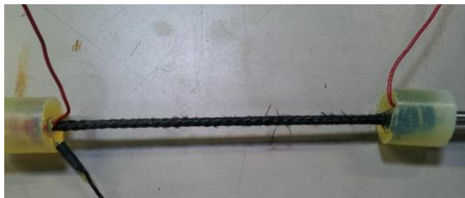
Figure 6. Photograph of Carbon Fiber Braided Tubular MEA
