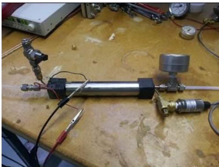
Figure 7. Photograph of a Single Tubular Reactor
